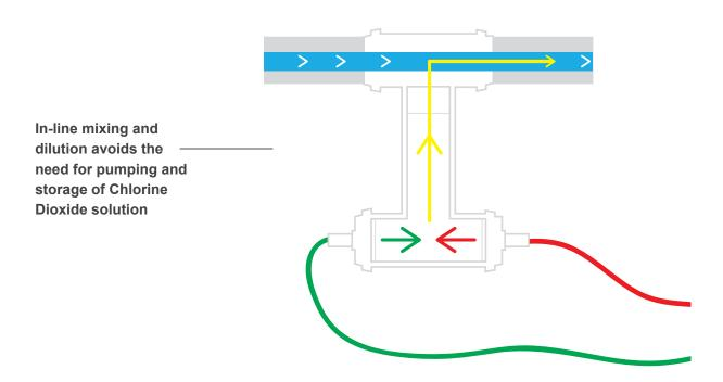
The Bravo WA™ is microprocessor controlled, and offers the ability to dose Chlorine Dioxide directly in proportion to the signals from an industry standard pulsed water meter. A variety of alarm inputs are provided, allowing for dosing to be started or stopped in response to alarm signals from customer processes, timers or stand-alone batch controllers.
