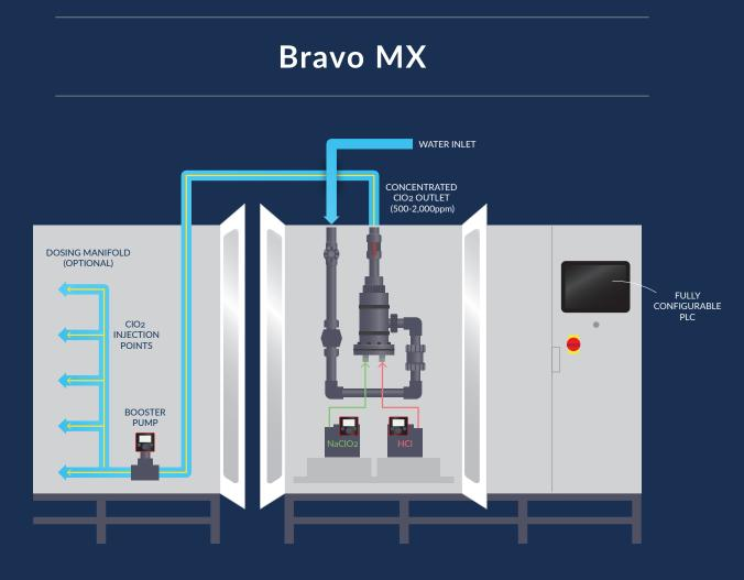
The Scotmas Bravo MX Chlorine Dioxide Generation and Dosing System is designed and built to comply with WIMES (Water Industry Mechanical and Electrical Specifications) requirements.
