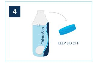
Fill the dilution bottle with cold water. Add ChloroSan tablets. The lid must be off until the tablets have completely dissolved. Dilute as per instructions below.
