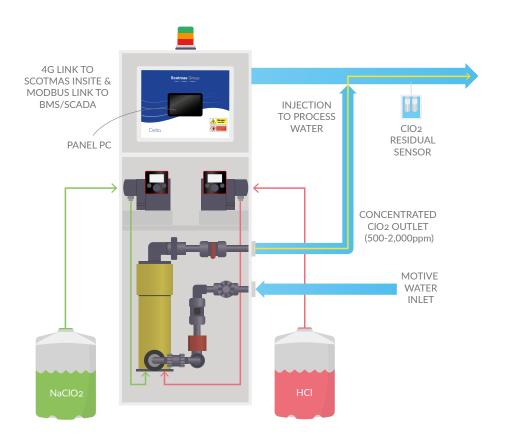
The Scotmas Delta WA Chlorine Dioxide Generation and Dosing System is designed to produce a stream of ClO2 solution for potable water, cooling tower dosing, wastewater treatment, food processing and other industrial applications.
