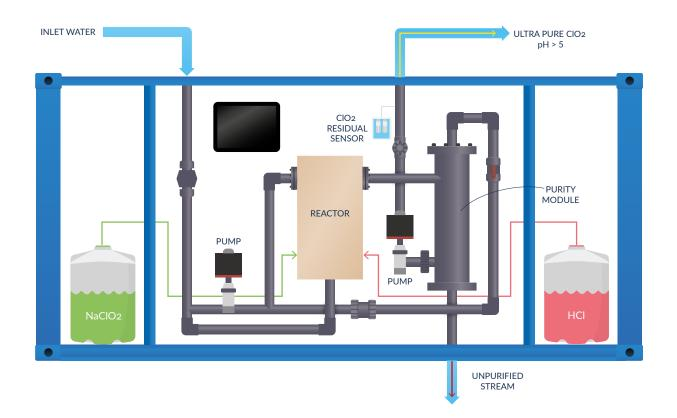
The Scotmas Bravo Ultra Pure Generation and Dosing System is a technology patented, WIMES (Water Industry Mechanical and Electrical Specifications) compliant system which introduces a stream of ultrapure Chlorine Dioxide solution (100% ClO2) into the treated water stream, without any other generation byproducts (GBP) from the reactor.
